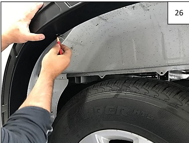
Align the flare on the fender and mark 3 holes using a grease pencil.
