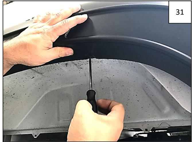
Start 3 supplied Truss-Head Screws through upper holes in flare and into clips installed in Step 29. Apply pressure to flare towards vehicle body at each fastening point and tighten all fasteners.
