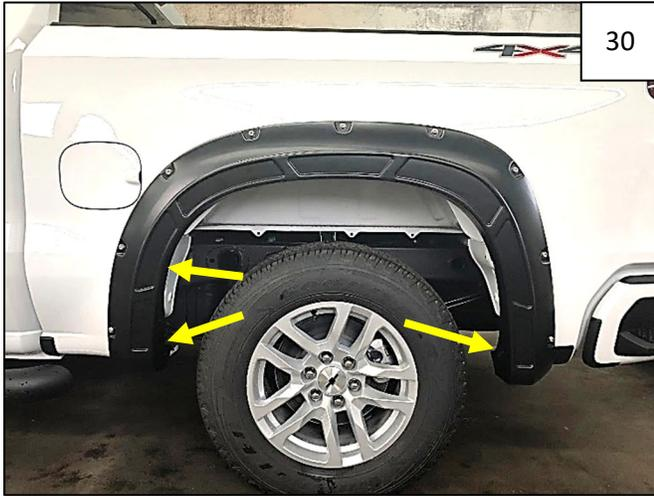
Hold flare on fender. Start 3 factory screws removed in Steps 24 and 25 as shown.
