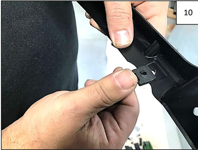
Attach 2 supplied Short "U" Clips to the supplied Inner Bracket as shown.
