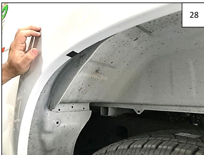
Peel liner from a supplied Foam Tab and center tab over each mark made in Step 26; fold each tab over lip of wheel well.
