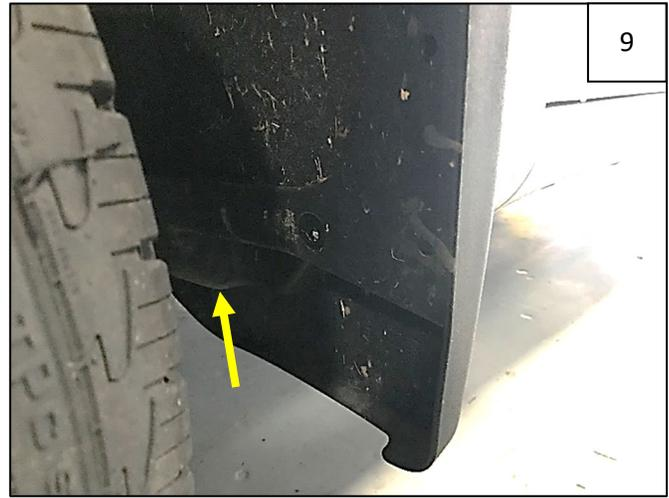
Using a 10mm socket, remove 1 factory bolt from mud flap indicated by arrow. Remove mud flap by pulling firmly away from vehicle body (a hidden clip will disengage).
