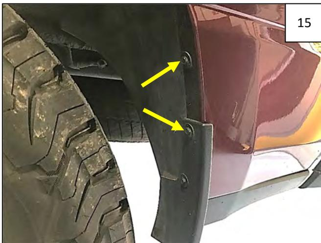
Using an 8mm socket, remove and retain 1 factory screw at top of rear mud flap. The mud flap will remain on the vehicle; do not remove any other mud flap fastener.
