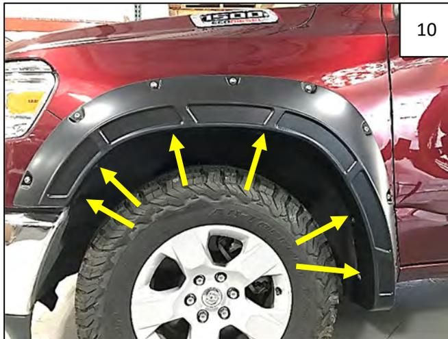
Align flare with vehicle. Start 6 factory screws through holes in flare and into factory holes.
