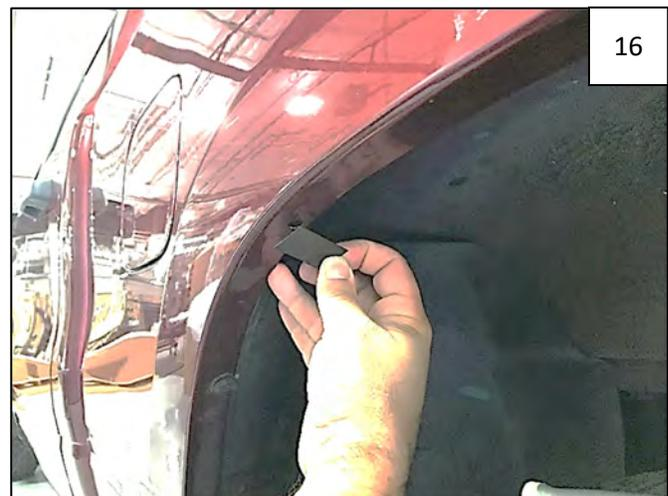
For 3 topmost holes in wheel well, peel liner from a supplied Mounting Tab and center over each factory hole (3 places).
