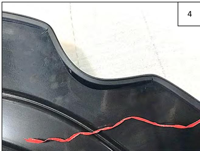
Correctly-installed edge trim around gas door.
