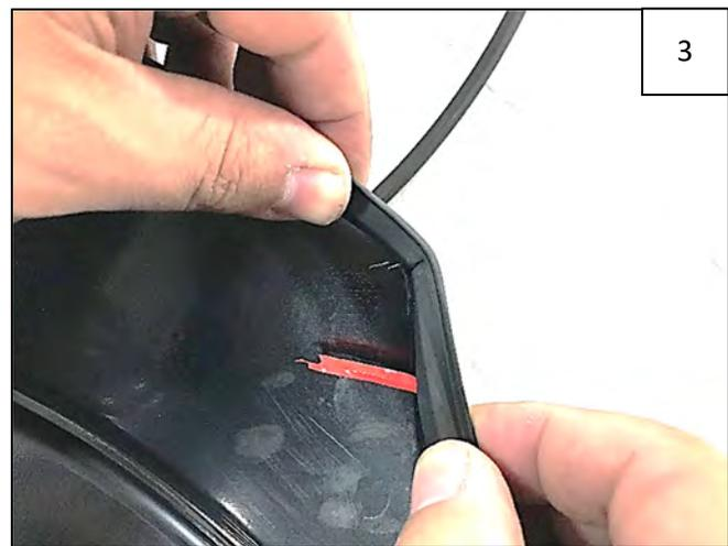
As you come to the second "point" in the flare, make another "V" notch in the backside of the edge trim, retaining 2-3 inches of vinyl backing. Proceed along the rest of the flare.
