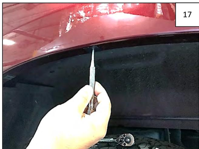
Using an awl, pierce Mounting tabs installed in Step 16 and into factory holes underneath.
