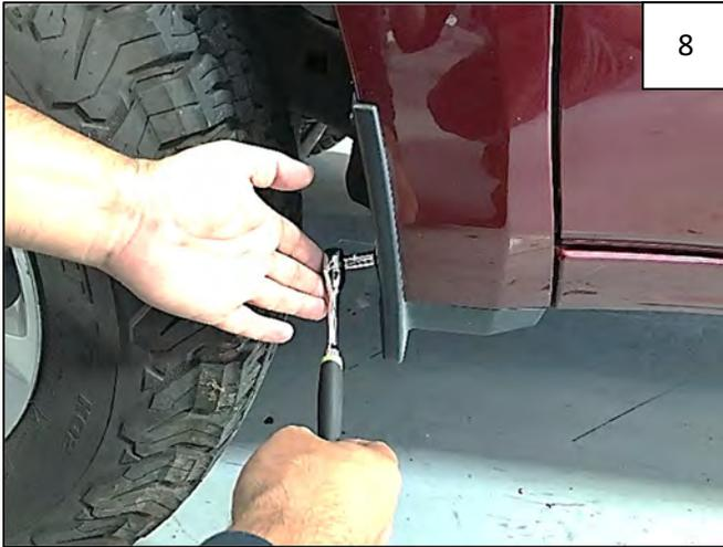
Remove 1 factory screw from center of mud flap. *The mudflap will remain on the vehicle – do not remove the other fasteners.*
