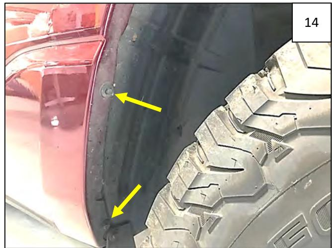
Using an 8mm socket, remove and retain 2 factory screws at front of rear wheel well.
