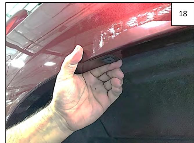
Slide a supplied "U" Clip over each Mounting tab, centering over holes made in Step 17 (3 places).
