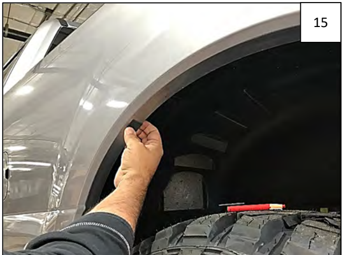
Peel liner from a supplied Foam Tab and center tab over each mark made in Step 13, folding each tab over the wheel well lip.
