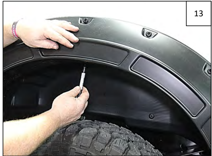
Align Rear Flare on fender using body style line and mud flap holes as a guide and mark 4 hole locations with a grease pencil.
