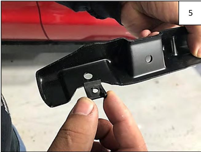
Attach 2 #14 "U" Clips to each Inner Bracket over pre-drilled holes as shown. **NOTE:** Driver Side Inner Bracket is marked with an "LF" and Passenger Side Inner Bracket is marked with an "RF."
