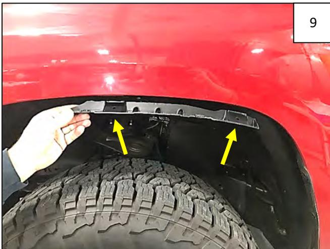
Using 2 supplied 20mm Hex Screws, attach Inner Bracket to factory holes with a 10mm socket (not at clip locations).
