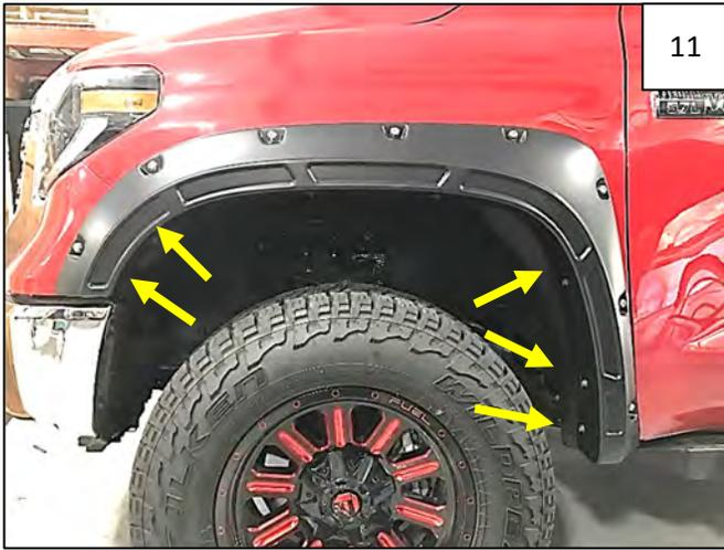
Start 3 supplied 20mm Hex Screws through the 3 rear holes in the flare and into factory holes in rear of Wheel well. Start 2 supplied 20mm Hex Screws through forwardmost holes in flare and into factory holes.
