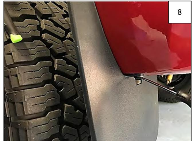
Using a pry tool or flathead screwdriver, remove plastic push retainer from underside of factory mud flap. Remove mud flap and discard.
