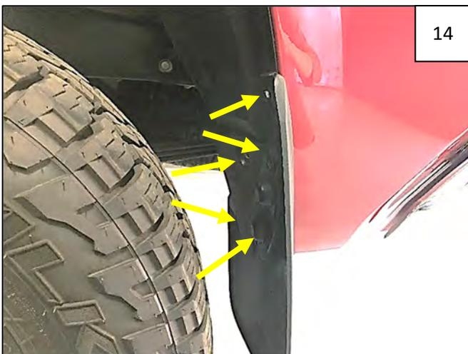
Using a 10mm socket, remove 5 factory screws attaching mud flap as shown.
