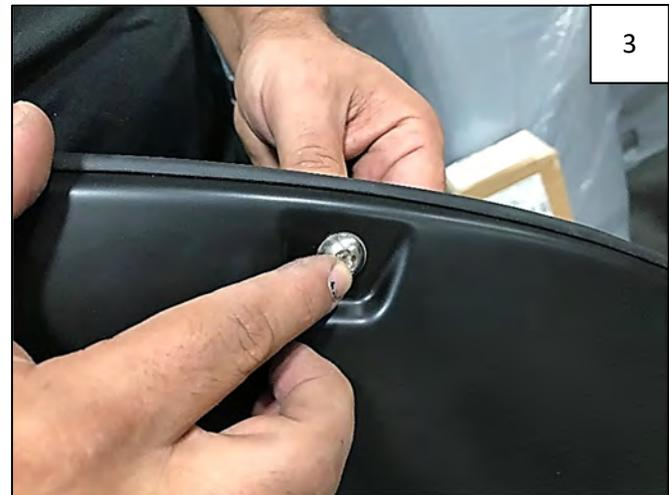
Insert each Bolt/Washer combination through pocket holes in flare, Bolt head and Washer on the outside.
