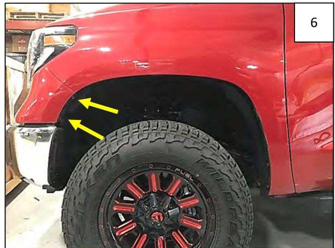
Using a 10mm socket, remove 2 factory fasteners from front of wheel well.
