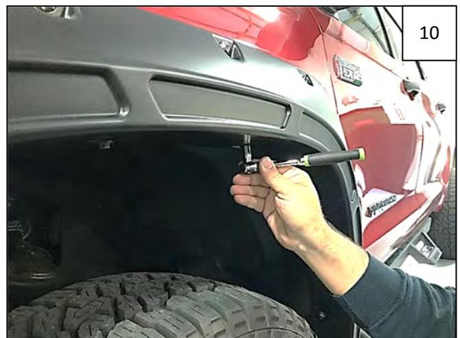
Hold flare on fender, pressing toward vehicle to align holes with clips installed in Inner Bracket in Step 5. Start 2 supplied 20mm Hex screws through top 2 holes in flare and into clips.
