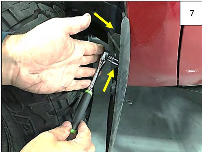
Using a 10mm socket, remove 2 factory fasteners from factory mud flap as shown.
