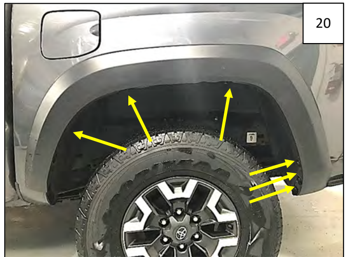
Remove 6 factory screws from factory flare as indicated by arrows. NOTE: If no factory flare is present, skip to Step 25.
