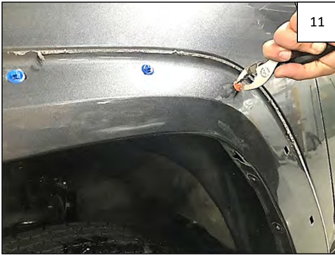
Use a vise grip or pliers to remove 1 factory clip as indicated by circle in Step 10, pulling with a rocking motion.
