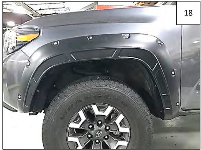
Complete Front Flare Installation.
