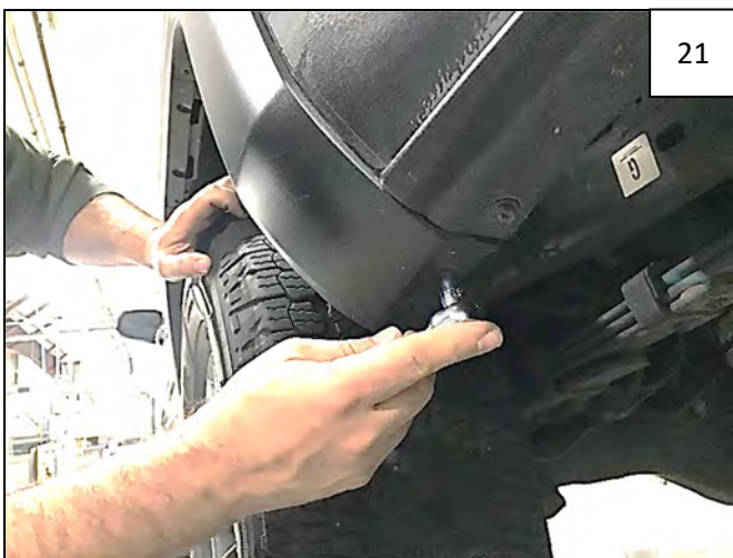
Remove 1 factory screw from underside of factory flare at rear.
