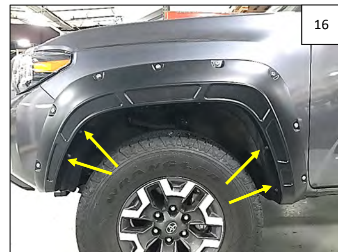
Install 4 supplied 20mm Hex Screws through remaining holes in flare and into holes in fender.
