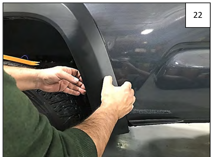
Remove factory flare by pulling firmly away from side of vehicle. Use a pry tool to protect paint if desired.
