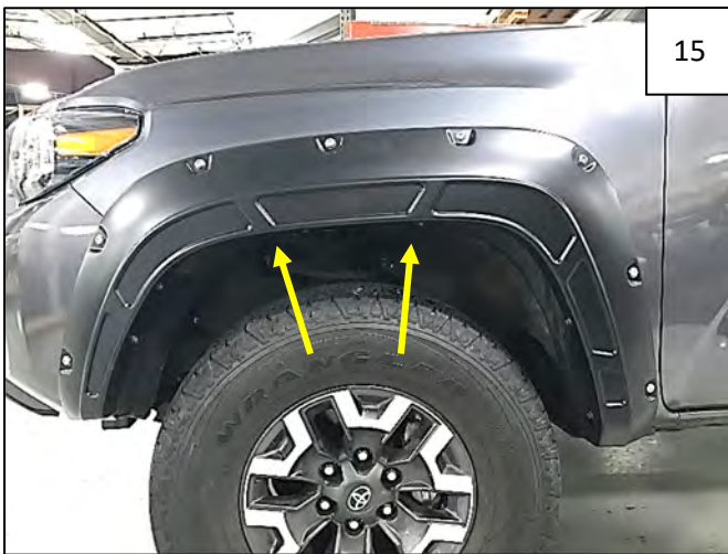
Aligning flare on fender and pressing toward vehicle, start 2 supplied 20mm Hex Screws through flare and into clips installed on Inner Bracket.
