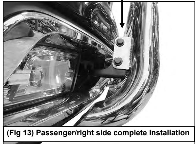
(Fig 13) Passenger/right side complete installation
