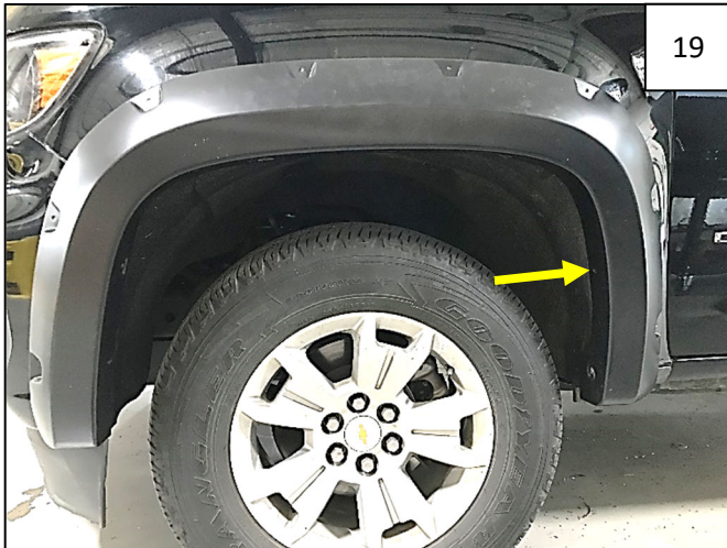
19 Hold flare on fender and start a supplied #10 Truss Head Screw through hole and into clip installed in Step 18. NOTE: Use an awl to locate and center hole in clip if needed.
