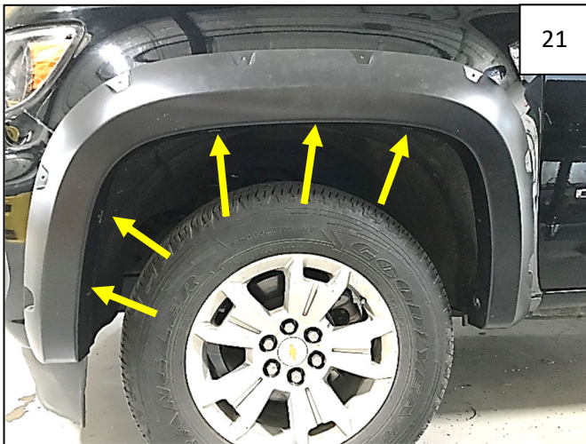
21 Install 5 supplied #10 Truss Head Screws through forwardmost holes in flare and into clips installed in the Long and Short Inner Pieces. NOTE: Use an awl to locate and center holes in clips if needed.
