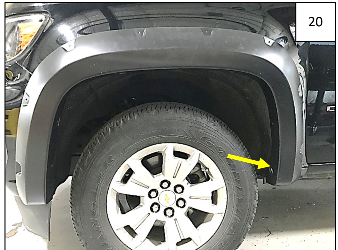
20 Install a factory screw through lowermost rear hole in flare and into factory hole in fender.
