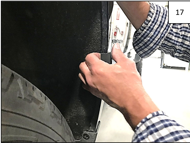
17 Peel PSA liner from supplied Mounting Tab. Center Mounting Tab on fender over mark made in Steps 15-16, folding over fender lip.
