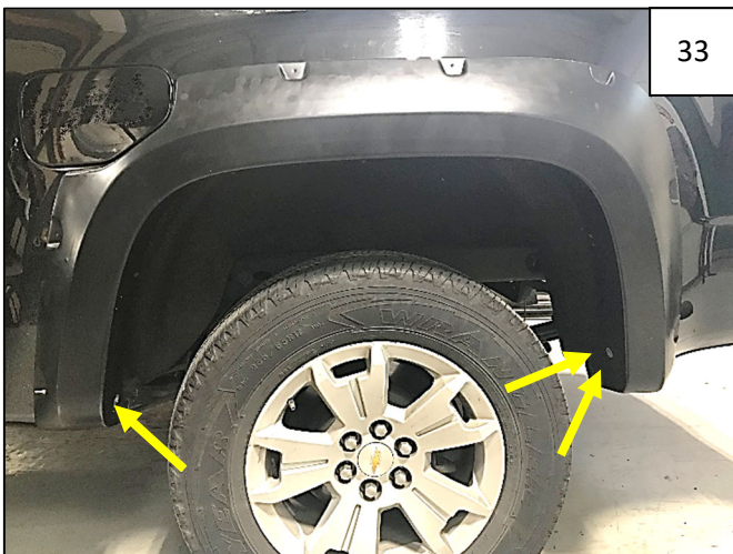
Hold flare firmly on fender. Start 3 factory screws in holes indicated by arrows.
