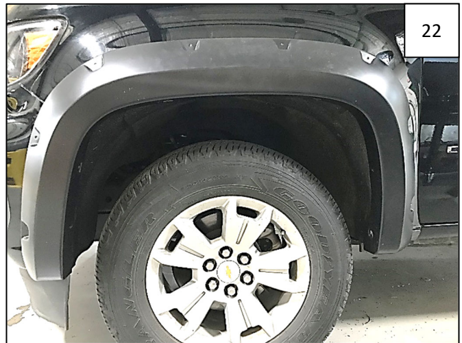
22 Apply pressure to outward face of the flare towards the center of the vehicle and tighten all screws.
