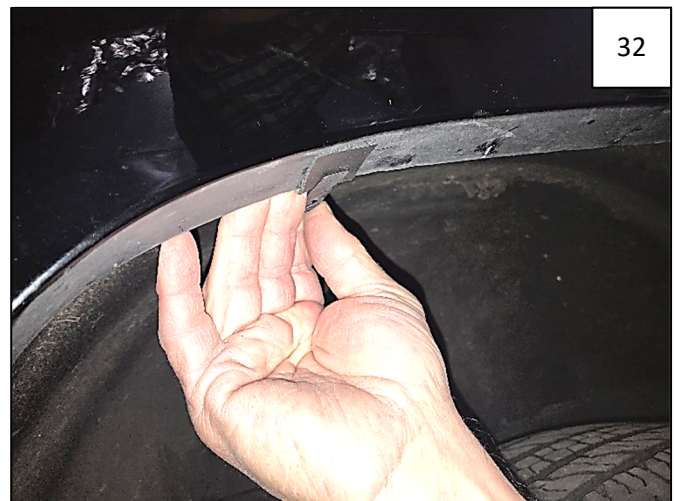
Slide a supplied Long "U" Clip over each Mounting Tab installed in Step 31.
