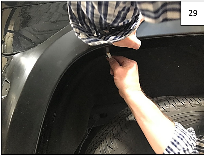
Hold flare firmly on fender. Using a grease pencil, mark 5 hole locations in area shown in Step 30.
