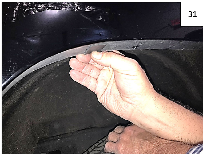
Center a supplied Mounting Tab over each mark made in Steps 29-30.
