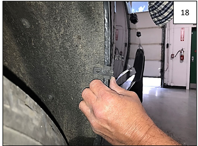
18 Slide a supplied Long "U" Clip over Mounting Tab.
