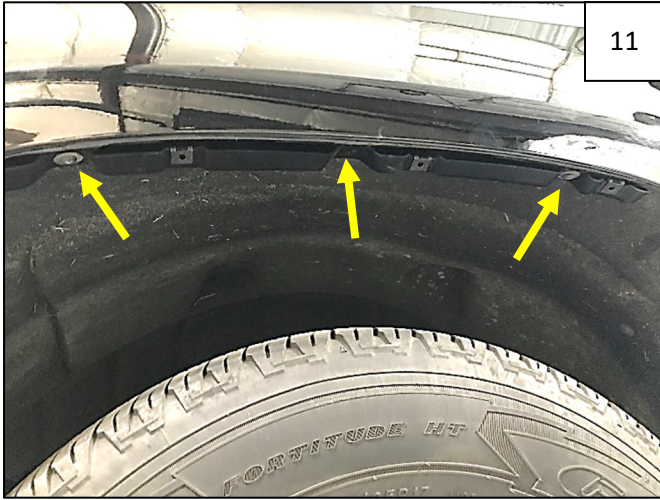
Install Long Inner Piece onto top underside lip of fender using 3 factory screws.
