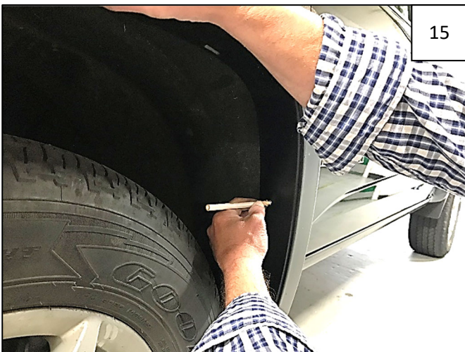
Hold flare firmly on fender. Using a grease pencil, mark 1 hole location in area shown in Step 16.
