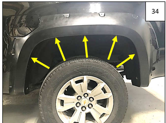
Start 5 supplied #10 Truss Head Screws through holes in flare and into clips installed in Step 32. NOTE: Use an awl to locate and center holes in clips if needed.
