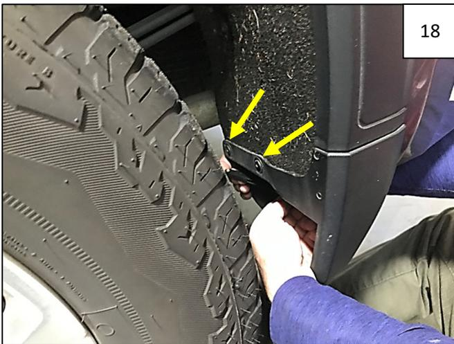
Remove 2 T-15 bolts from mud guard at inside rear of wheel well.
