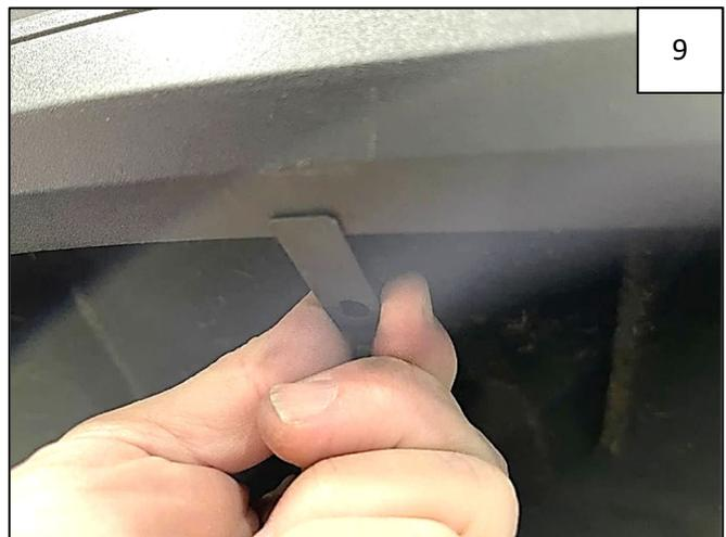
Remove flare from fender and slide a supplied "U" Clip over plastic lip in 4 locations, centering over marks made in Step 8.
