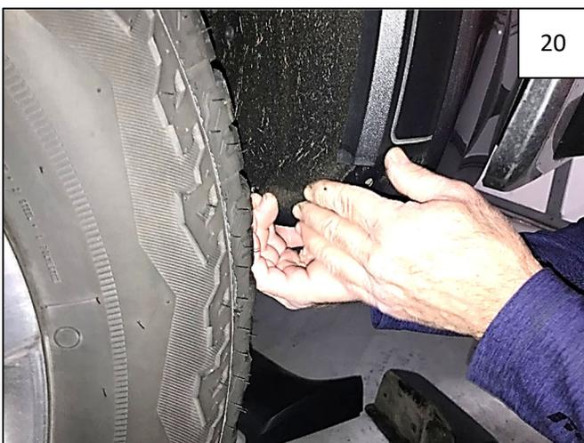
Tuck factory splash shield into fender sheet metal lip at both front and rear of wheel well. The sheet metal lip will need to be accessible for clip installation in Step 24.
