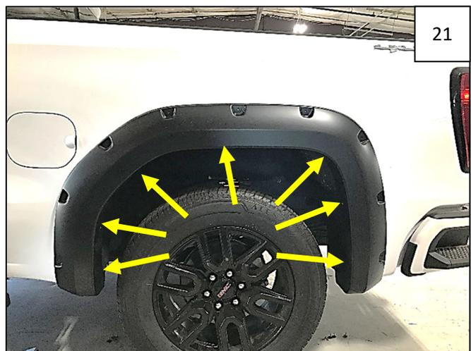
Hold flare firmly on vehicle. Using a grease pencil, mark 7 hole locations through flare onto fender lip.
