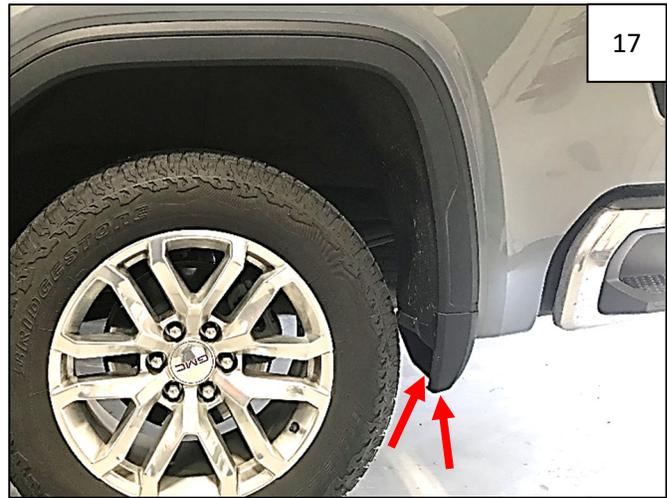
At rear of rear wheel well, remove 2 T-15 bolts from underside of rearward mud guard.
