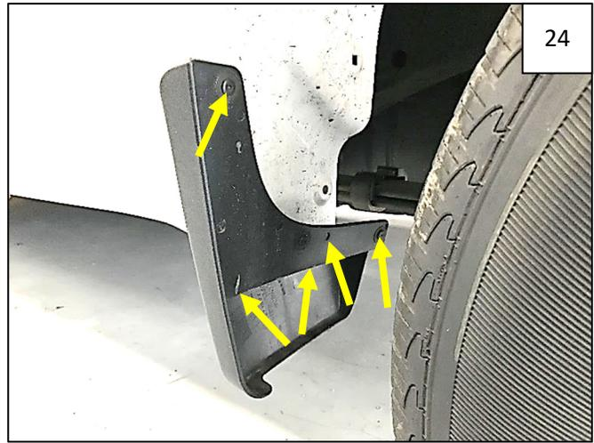
Remove 5 factory screws from the front splash guard. Splash guard is held on with a hidden clip – to remove, pull splash guard firmly from vehicle.
