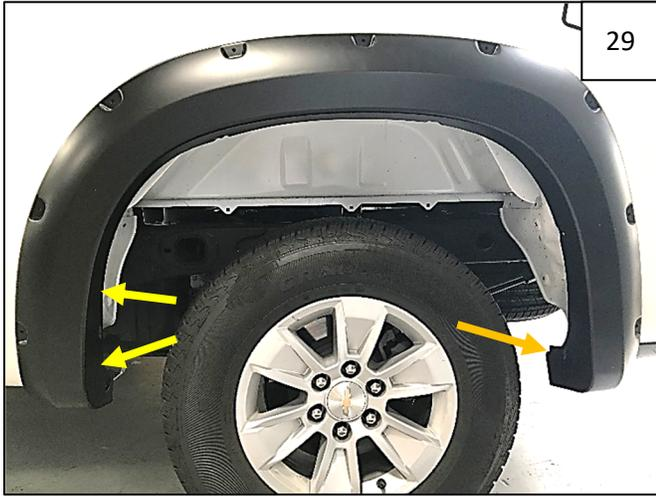
Hold flare on fender. Start 3 factory screws removed in Steps 23 and 24 as shown.
