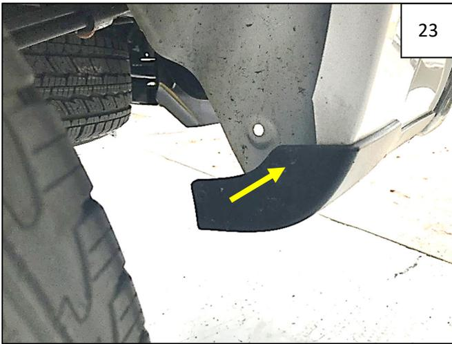
Remove 1 factory T15 Torx screw on rear splash guard. Retain all factory screws; some will be used.
