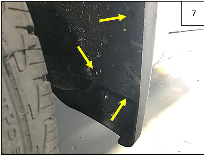
Using a T15 Torx bit, remove 3 factory fasteners indicated by arrows holding the factory mud flap on. Retain all screws.
