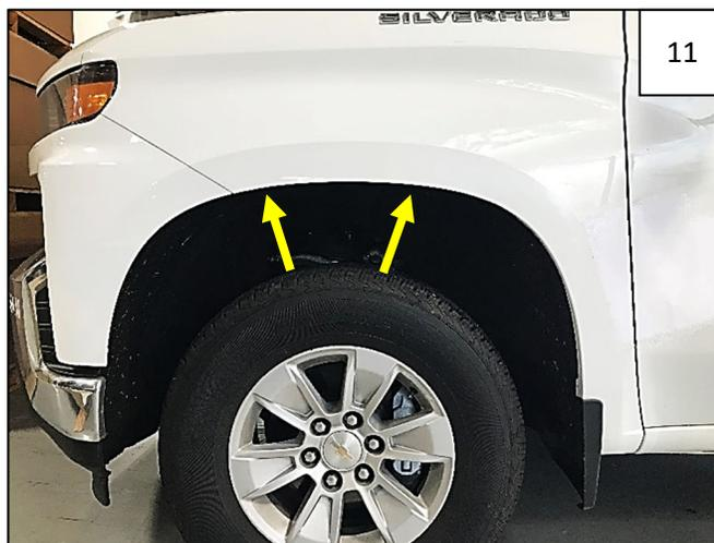
Remove 2 factory T15 Torx screws at top of wheel well as shown. Retain.
