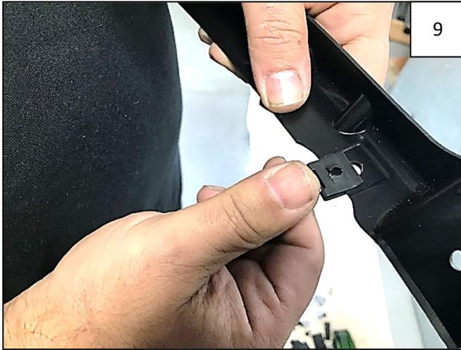
Attach 2 supplied Short "U" Clips to the supplied Top Inner Bracket as shown.
