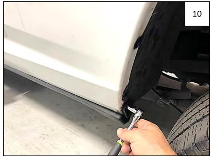
Using an 8mm socket, remove and retain factory screw at front of rear wheel well.
