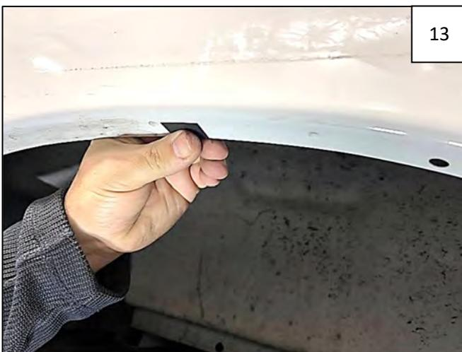
For topmost hole in wheel well, peel liner from a supplied Mounting Tab and center over the factory hole. If vehicle had full wheel well liners, no tab or clip is needed – just reuse factory fastener.
