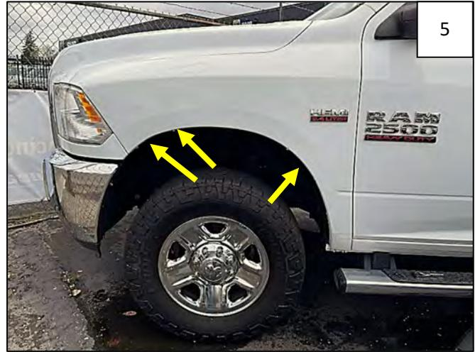
Remove and retain 3 factory screws as shown.
