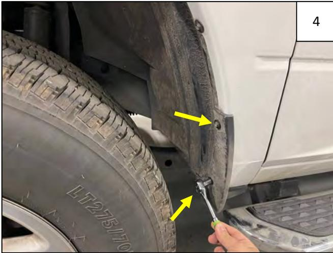
Remove 2 factory screws from mud flap. Fasteners will be reused. Do not remove fastener above mud flap. Pull mud flap towards you to remove – it's held on with 2 hidden plastic clips.
