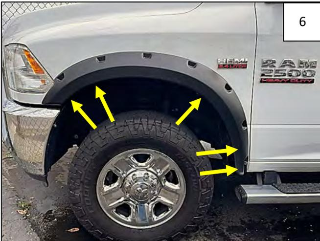
Align flare with vehicle. Start 5 factory screws through holes in flare and into factory holes.
