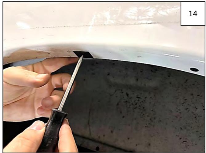
Using an awl, pierce Mounting Tab into the factory hole underneath.
