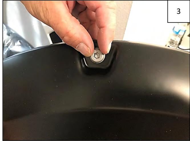
Insert Push-In Pocket Hardware into each flare pocket hole (on outer flare surface, 8 places each front flare, 9 places each rear flare). Push in to engage clip and tape adhesion.
