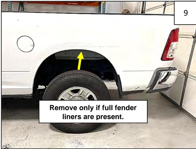
If vehicle is equipped with full fender liners, remove top most factory screw at top of fender; retain for reuse. If vehicle is not equipped with fender liners, proceed to Step 10.
