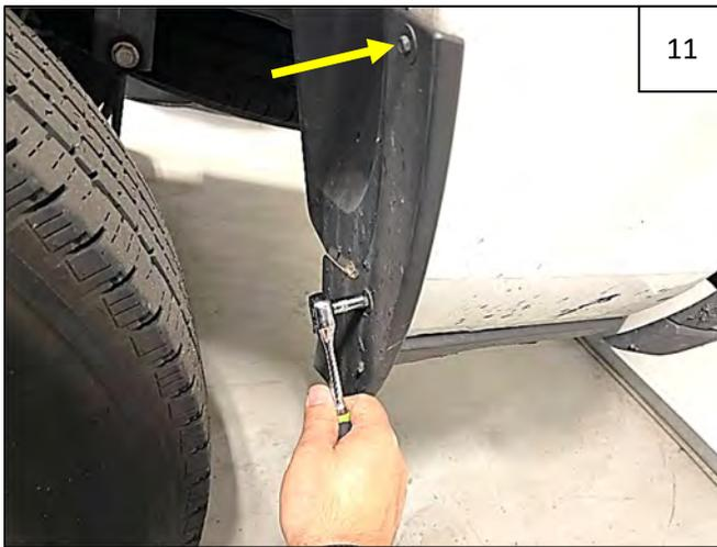
Using an 8mm socket, remove 2 fasteners at rear mudflap. Retain factory screws. Pull until plastic clips release.
