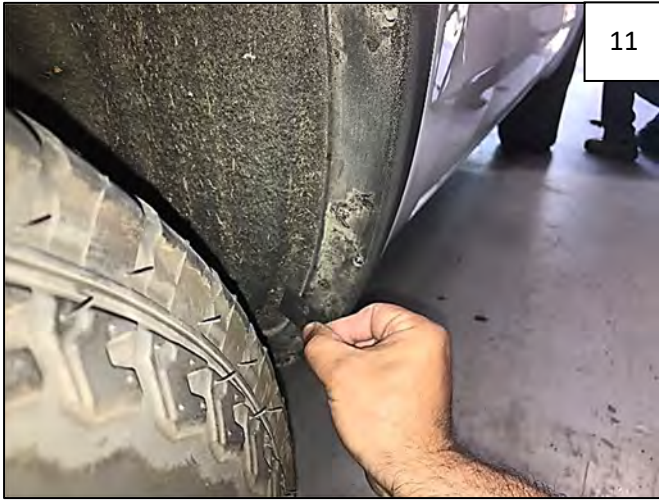
Peel PSA liner from supplied Mylar Tab. Center Mounting Tab on fender over mark made in Steps 9-10, folding over fender lip.
