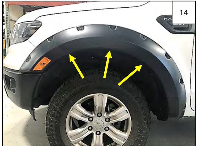
Hold flare firmly on fender, and install 3 supplied Plastic Push-In Retainers through holes in flare and into fender where indicated.
