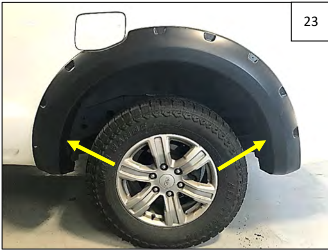
Install a supplied Long Screw through flare and into each clip installed in Step 21.
