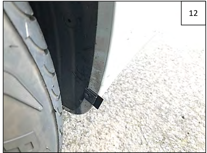
Slide a supplied "S" Clip over Mylar Tab and fender lip.
