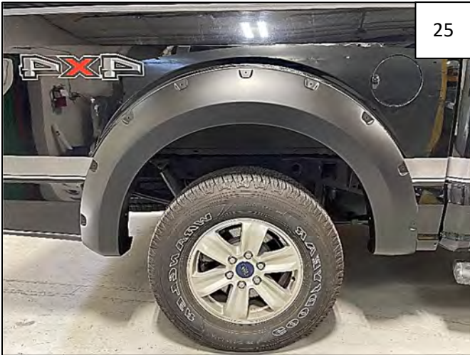
Completed rear flare installation.
