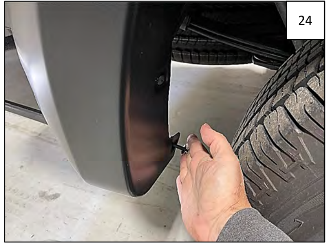
Install supplied Nylon Retainer through flare and into factory hole at rear of wheel well.
