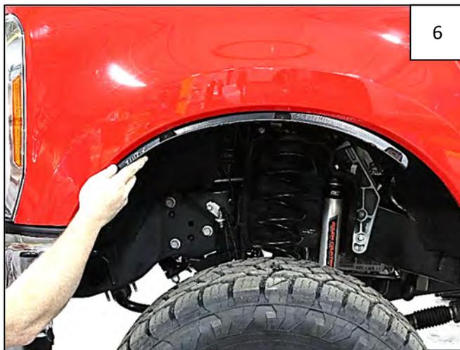
Line up holes in the Inner Bracket with the 4 upper-most factory holes in wheel well.
