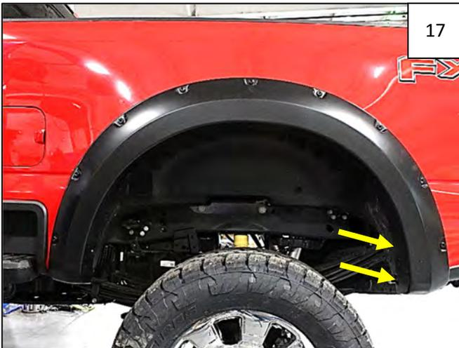
Install 2 supplied Plastic Retainers through flare and into factory holes at rear of wheel well.
