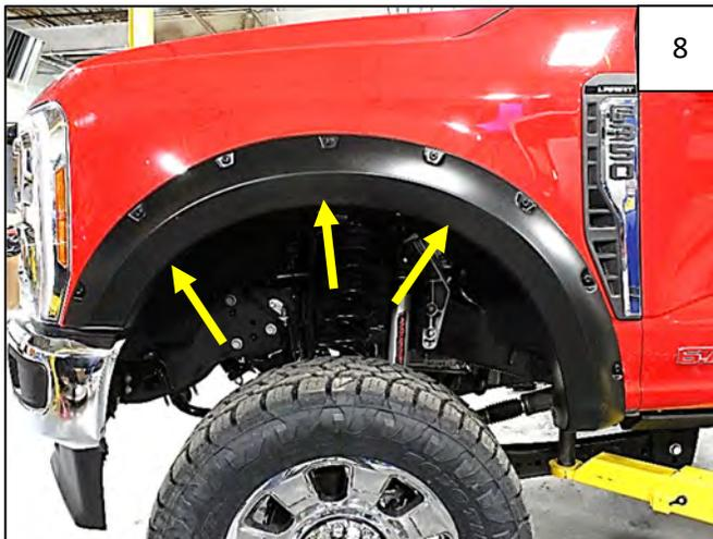
Aligning flare on fender, press inward on the flare to line up the flare mounting holes with the clips on the Inner Bracket. Install 3 supplied Truss-Head Screws through the flare and into the inner piece. Do not tighten.
