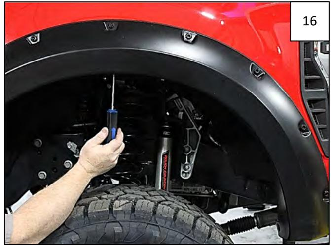
While holding flare to vehicle, start supplied Truss-Head Screws through the 4 topmost mounting holes in flare and into clips installed in Step 15. Apply pressure to flare towards vehicle body at each fastening point and tighten all fasteners.
