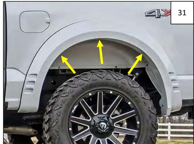
Install 3 supplied #10 Truss-Head Screws through upper holes in flare and into clips installed in Step 29. Apply pressure to flare towards vehicle body at each fastening point and tighten all fasteners.
