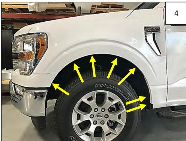
If your vehicle is 2021-2023, use 7mm socket to remove 7 factory screws from wheel well. Retain all screws for reinstallation.
