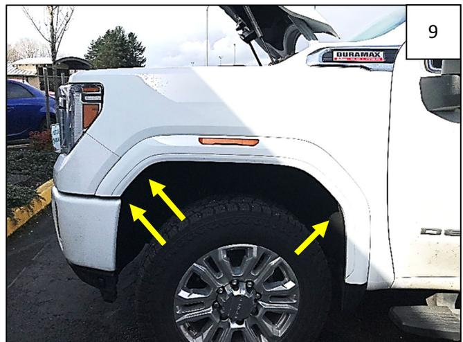
Remove 3 T-15 Torx screws from inside wheel well at locations shown.
