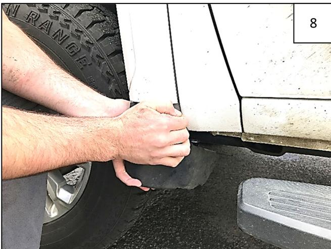
Remove mud guard by prying down and away from vehicle body, disengaging one internal clip. Discard mud guard.
