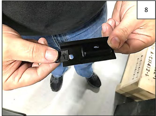
Slide a supplied Short "U" Clip onto plastic Inner Piece as shown.
