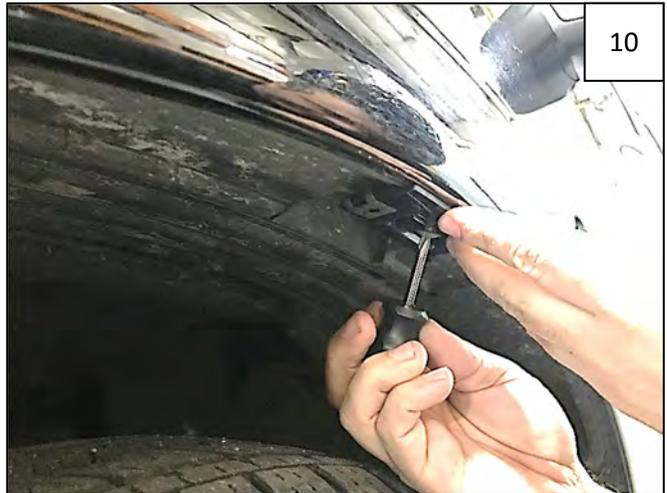
Install Inner Piece in fender well using factory screw removed in Step 9, at location in same location it was removed from (do not use clip hole to install Inner Piece).
