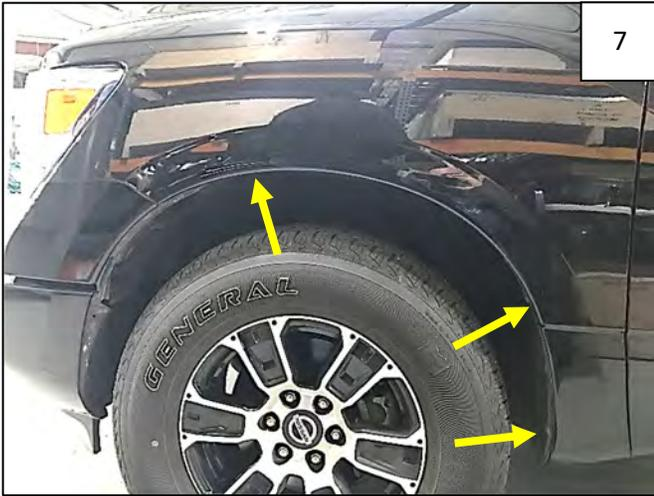
Using a Phillips screwdriver, remove 3 factory screws at locations shown. NOTE: in the tight wheel well, it is helpful to use a stubby screwdriver. Retain all screws.
