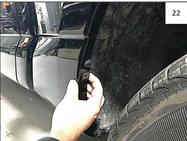
Slide a supplied Short "U" Clip over Plastic Mounting Tab installed in Step 20.
