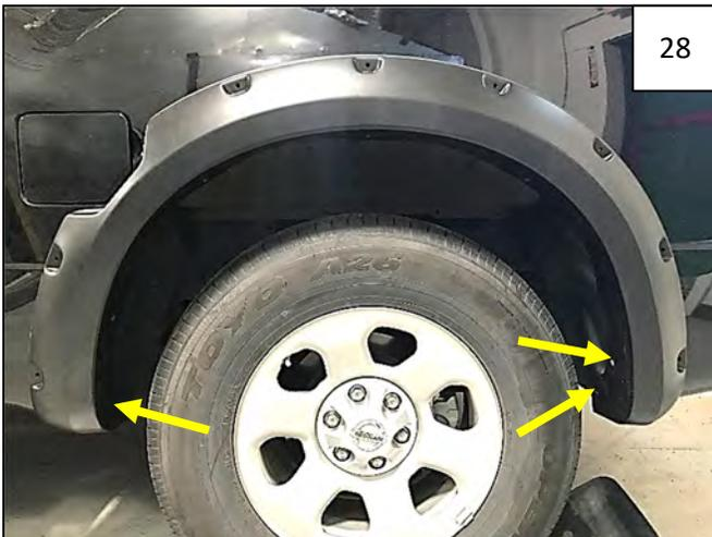
Reposition flare on fender. Start 3 factory screws in lower holes indicated by arrows.
