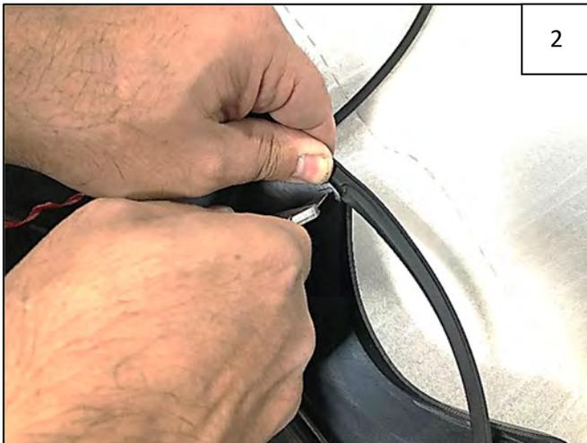
As you come to the first "point" of the flare, cut a "V" notch into the backside of the edge trim at the sharpest part of the curve. Make sure that you retain 2-3 inches of vinyl backing for ease of further installation.
