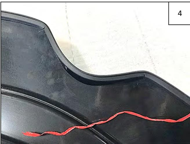
Correctly-installed edge trim around gas door.
