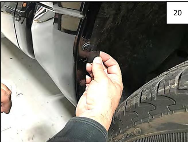
Peel liner from supplied Plastic Mounting Tab. Center tab over square hole in fender lip located at area shown in Step 21. Fold tab over fender lip.
