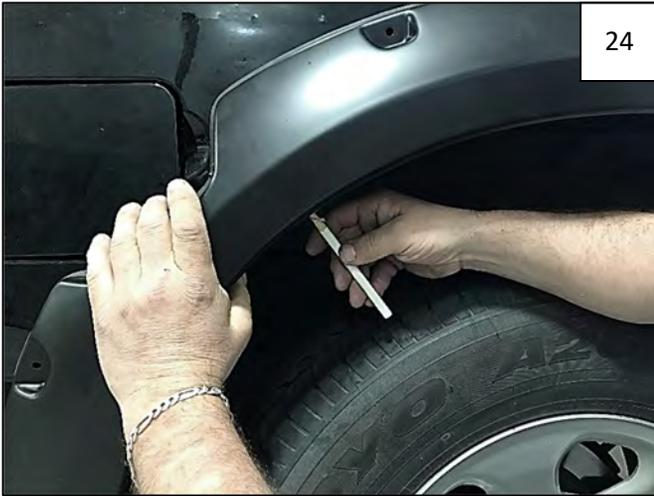
Hold flare firmly on fender and mark 3 hole locations at arrows shown in Step 25.
