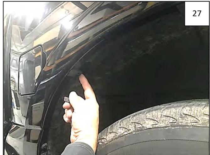
Slide a supplied Long "U" Clip over each tab, centering approximately over mark made in Step 24.
