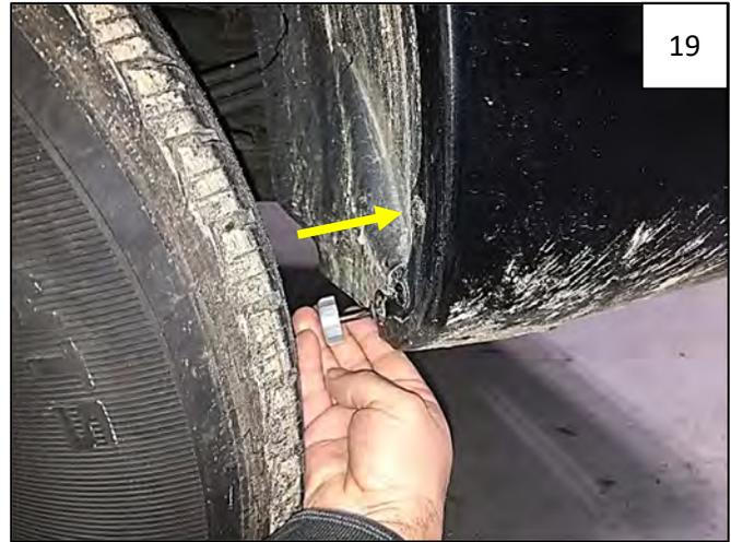
Remove 2 factory screws from rear of rear wheel well.
