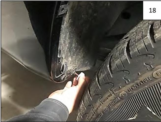
Remove 1 factory screw from front of rear wheel well. Retain all screws.
