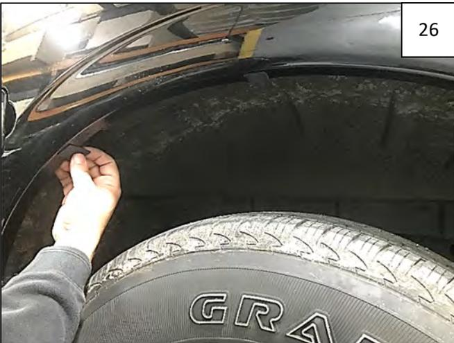
Peel liner from supplied Foam Mounting tab. Center a tab over each mark made in Step 24.
