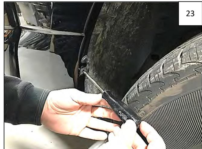
Use an awl to poke hole in Mounting tab, through screw hole in clip.
