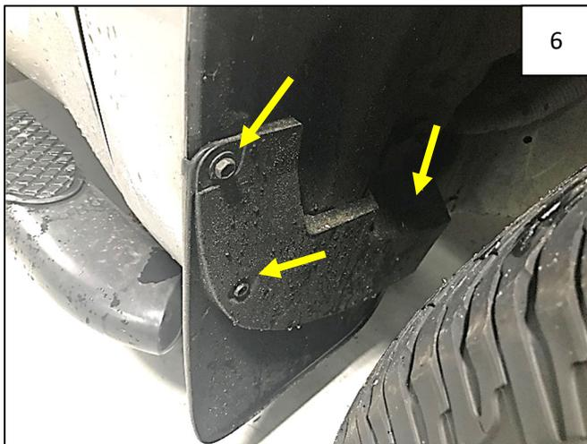
Using a 10mm socket, remove 3 factory fasteners from factory mud flap as shown.
