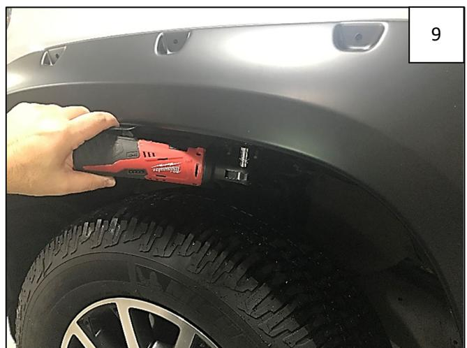
Hold flare on fender, pressing toward vehicle to align holes with clips installed in Inner Bracket in Step 4. Start 2 supplied 20mm Hex screws through top 2 holes in flare and into clips.
