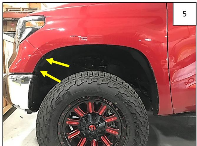
Using a 10mm socket, remove 2 factory fasteners from front of wheel well. **NOTE:** Screws are engaged in factory clips – do not remove clips.
