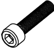
M6 x25 Socket Cap Screw x8
