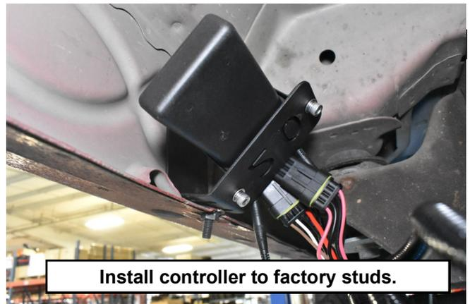
8. Connect the corresponding electrical connectors of the main harness to the controller. **Photo 7 / 8**
