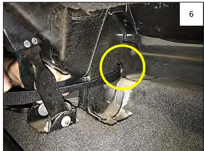
Loop other Safety Strap between seat belt sheaths and through 1" hole in strut under rear passenger side seat as shown.
