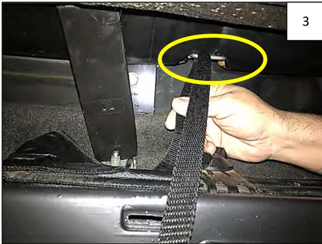
Loop one Safety Strap around metal loop located at underside of rear driver side seat.
