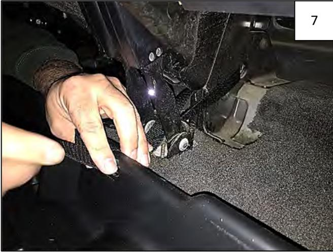
Feed Safety Strap through passenger side slot in Underseat Storage Box. Thread one Buckle on one end of Safety Strap.
