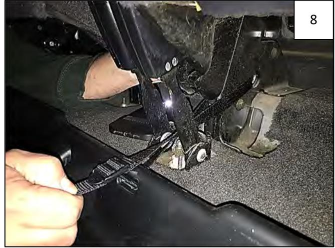
Feed other end of Safety Strap into Buckle and tighten.
