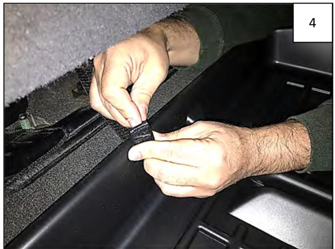
Feed a Safety Strap through driver side slot in Underseat Storage Box. Thread one Buckle on one end of Safety Strap.
