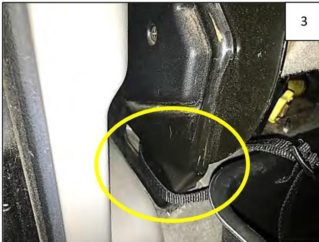
Loop each Safety Strap around seat strut on each end of seat near door.
