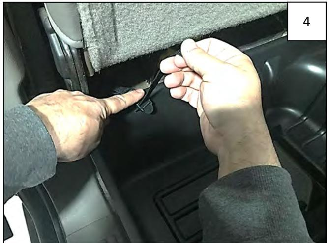
Feed a Safety Strap through each slot in Underseat Storage Box. Thread one Buckle on one end of Safety Strap.
