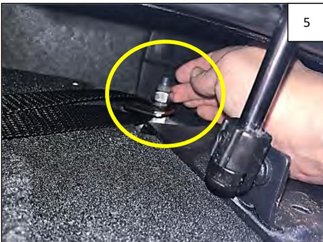
Thread a supplied Flange Nut onto each bolt. The nut does not need to be wrench-tight, but should be securely threaded down to the Metal Bracket.
