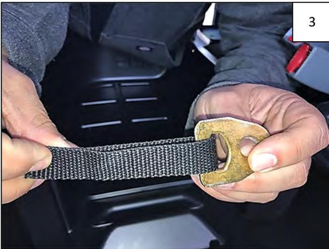
Feed one Safety Strap through the wide slot in each supplied Metal Bracket.
