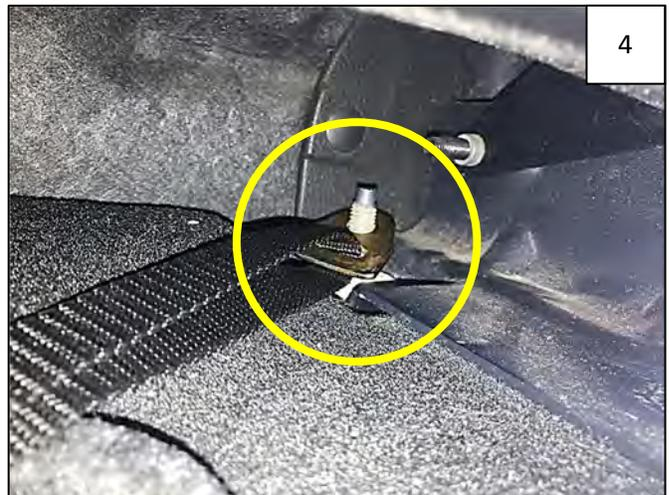
Slide a Metal Bracket-Step combo over each upright bolt located underneath seat closest to slots in rear of Underseat Storage Box.
