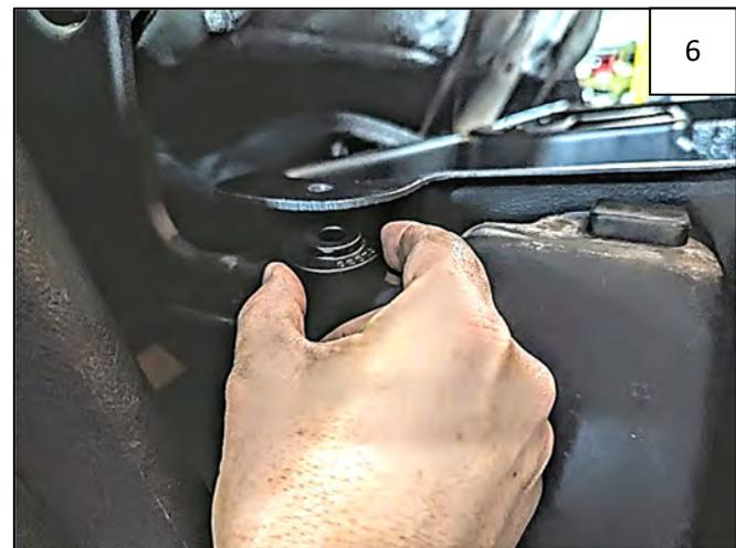
Slide a supplied Bushing between Underseat Storage Box and Clip.
