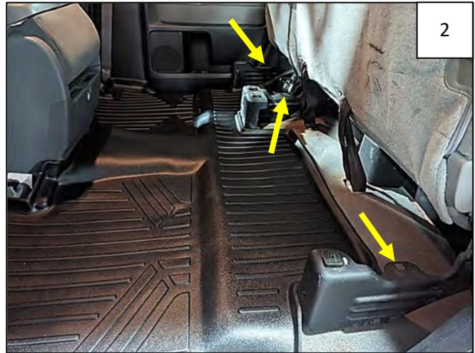
Slide 3 supplied Body Clip Nuts over square holes in seat support brackets indicated by arrows.
