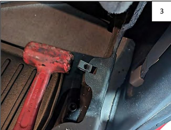
Use a deadblow/rubber hammer to align hole in clip with square hole.
