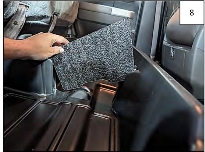
Install Passenger Side Foam Divider into molded-in slot in Underseat Storage Box.
