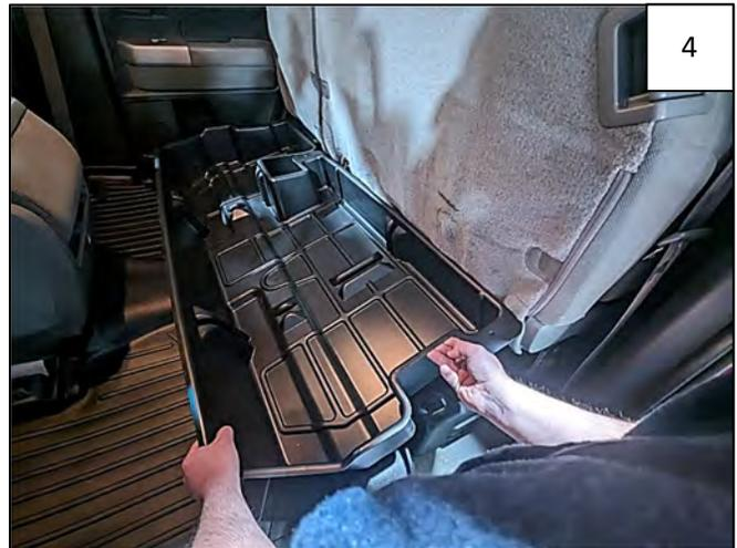
Place the underseat Storage Box on the floor, aligning holes in Box with clips installed in Steps 2-3.
