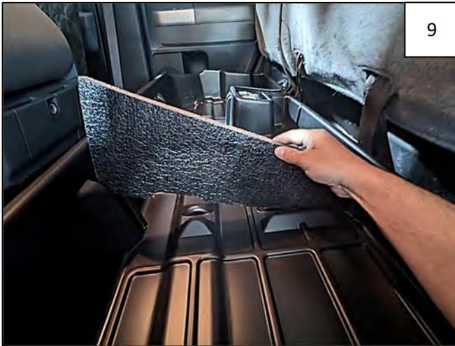
Install Driver Side Foam Divider into molded-in slot in Underseat Storage Box.
