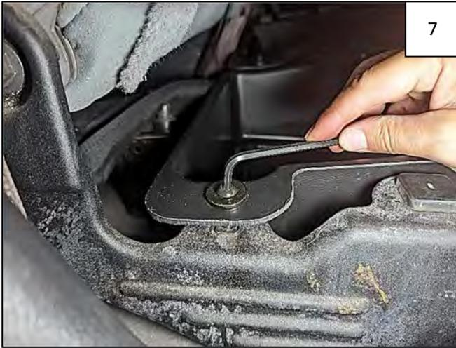
Holding bushing in place, insert Buttonhead Bolt through hole in Underseat Storage box and Bushing and thread into clip. Use a 3/16" Allen Wrench to tighten.
