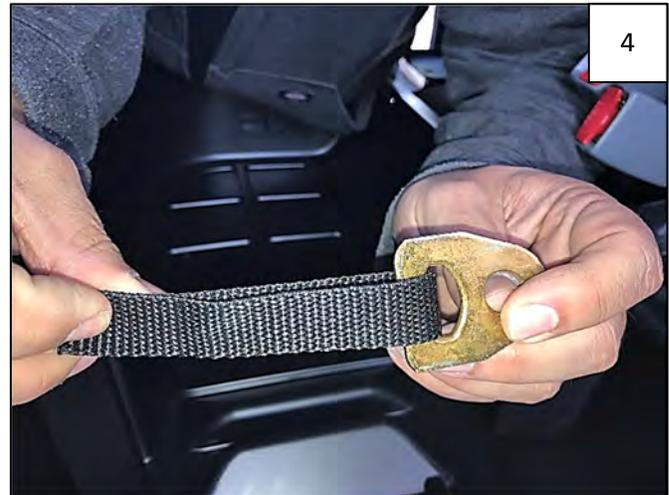
Feed Safety Strap through the wide slot in the supplied Metal Bracket.
