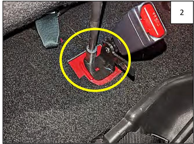
Using a 14mm socket, remove bolt at base of seat belt bracket under seat (1 place).
