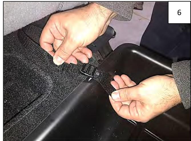
Thread buckle onto one end of safety strap. Feed other end of Safety Strap into Buckle and tighten to anchor Underseat Storage Box in place.
