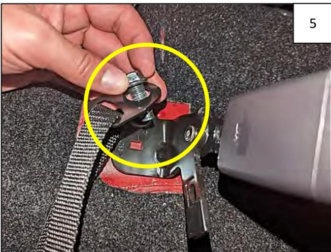
Slide Metal Bracket-Strap combo over bolt removed in Step 2. Reinstall bolt.
