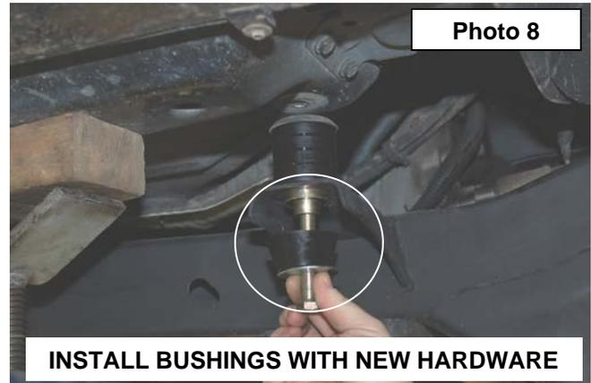
17. Install the lower bushing / crush sleeve and washer in the 4 rear mounts. Apply thread locker to the supplied 7/16" x 4" bolts and install. Do not tighten at this time.
