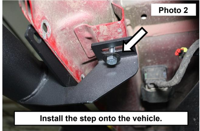
3. Install the (2) of the supplied 8mm-1.25 x 25mm Hex Head Bolts and (4) 8mm Flat washers and (2) 8mm-1.25 nuts in to the (3) pinch weld mounts. **Use included shims for front or rear mounts to fill gap if needed. Do NOT use the shims in the middle mount.** See Photo 3.
