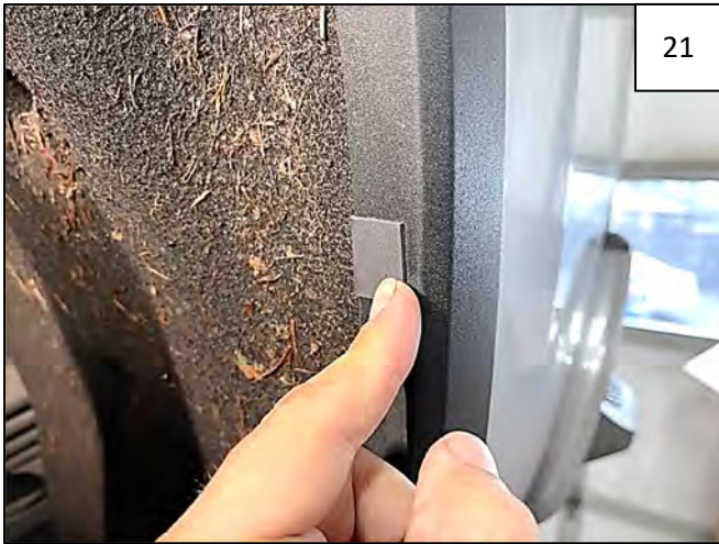
Peel liner from a supplied Foam Tab and center tab over each mark made in Step 19, folding over lip of wheel well.
