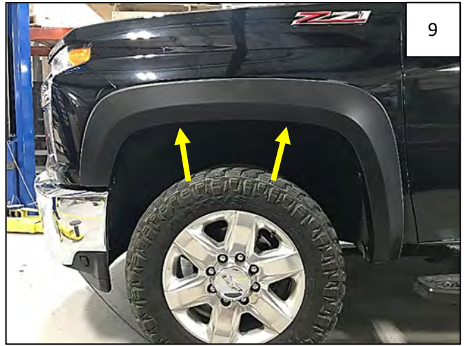
Align flare on vehicle and install 2 supplied Truss-Head Screws into clips on Inner Bracket as indicated by arrows.
