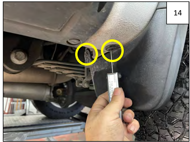
Remove 2 factory screws from underside of splash guard. Remove and discard factory splash guard.
