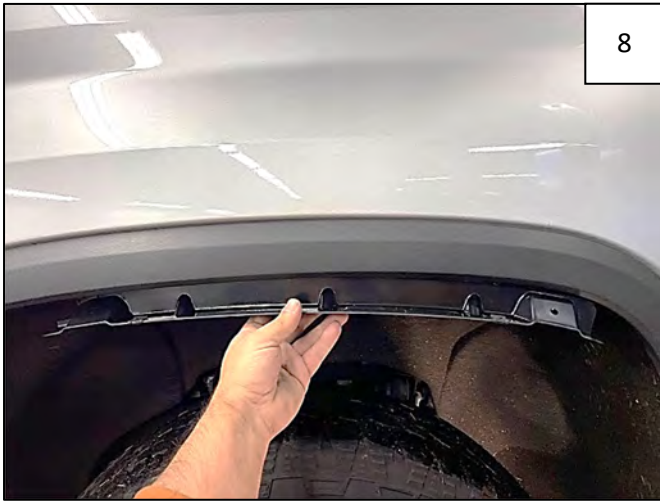
Install Inner Bracket using 2 T15 Torx screws retained in Step 7. Tighten both fasteners.
