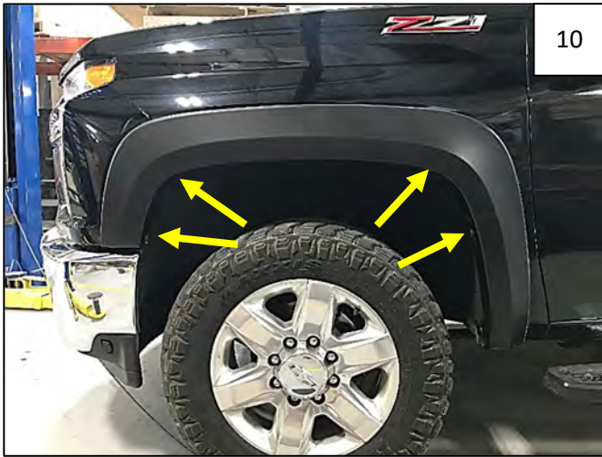
Reinstall 4 factory screws through holes in flare and into holes in fender.
