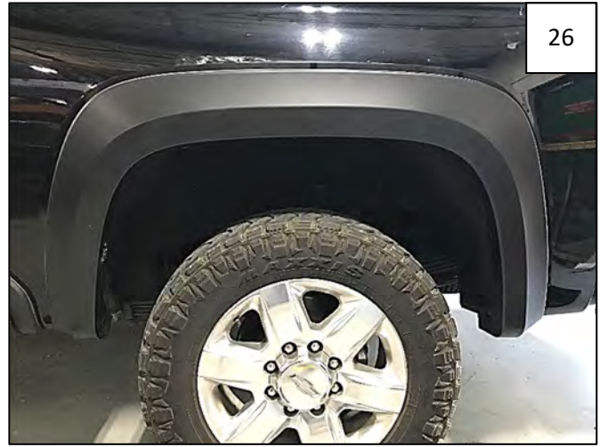
Completed Rear Flare installation.
