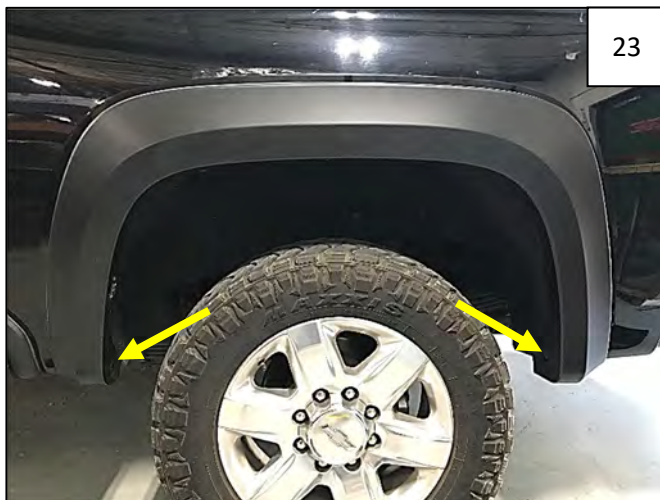
Hold flare on fender. Start 2 factory screws removed in Steps 13 and 15 as shown.
