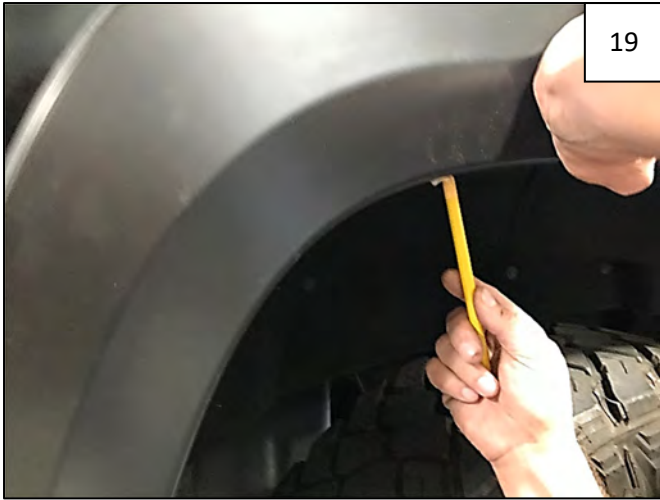
Hold the flare on the fender and mark 5 holes using a grease pencil.
