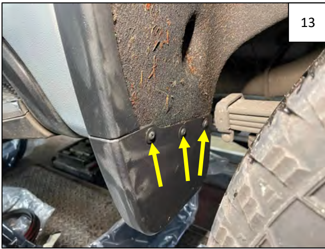
Remove 3 factory T15 Torx screw on the forward rear splash guard. Retain all factory screws; some will be used.
