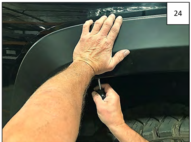
Start 3 supplied Truss-Head Screws through upper holes in flare and into clips installed in Step 22. Use an awl to locate clip holes as needed.
