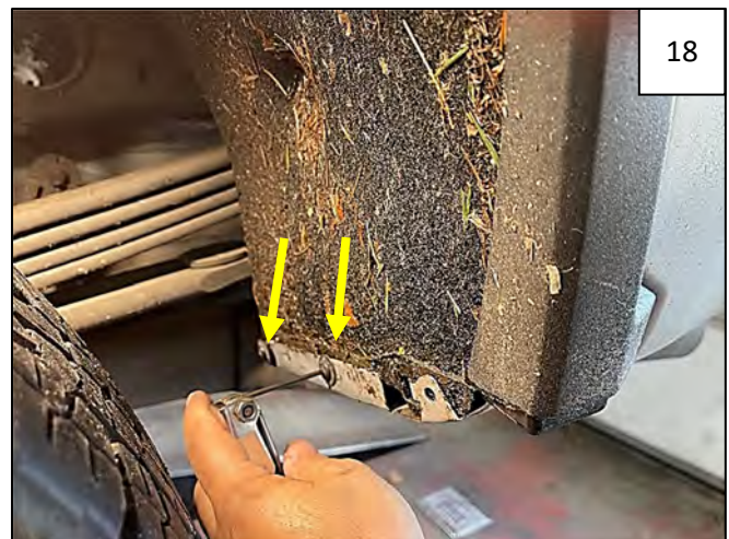
Reinstall 2 factory screws in rear of wheel well as shown to keep wheel well liner in place (outermost hole will be used in the flare installation).
