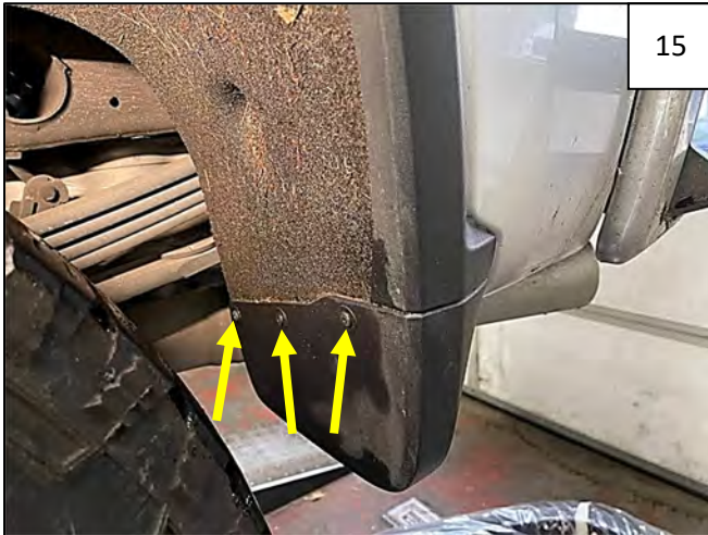
Remove 3 factory screws from the rearward rear splash guard.
