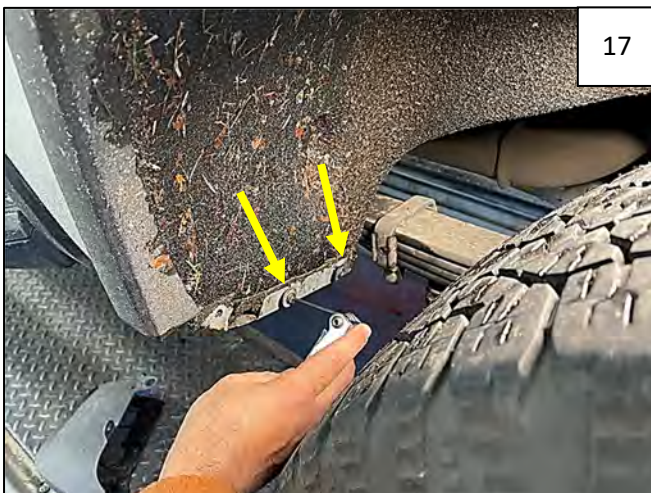
Reinstall 2 factory screws in front of wheel well as shown to keep wheel well liner in place (outermost hole will be used in the flare installation).
