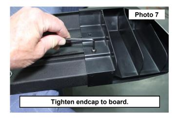
**SANITY CHECK**: Before moving to installation, the following should be complete. All four tread plates are fastened, Qty 3 of the 6MM hex bolts are in each of the T-slot rails, and the end caps are bolted into place? If the answer is **YES** to all of these, proceed to vehicle installation. If you answered **NO** to any of these, stop drinking and call a friend to help, or find a local installer to correct your mistakes.
