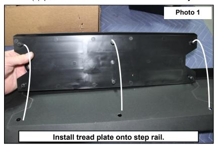
**Step 1:** Place the molded tread-plate onto the running board aligning the pegs with the holes in the step board **(Photo 1)**. These pegs will protrude through the step board. The self threading nuts will then be used to secure the tread-pate onto the step board.
