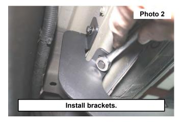
3. Align the bolts in the track of the assembled step boards with the slots of the brackets. Use the supplied 6mm washer and lock nut to secure. Use a 10mm wrench to tighten. **See Photo 3.**
