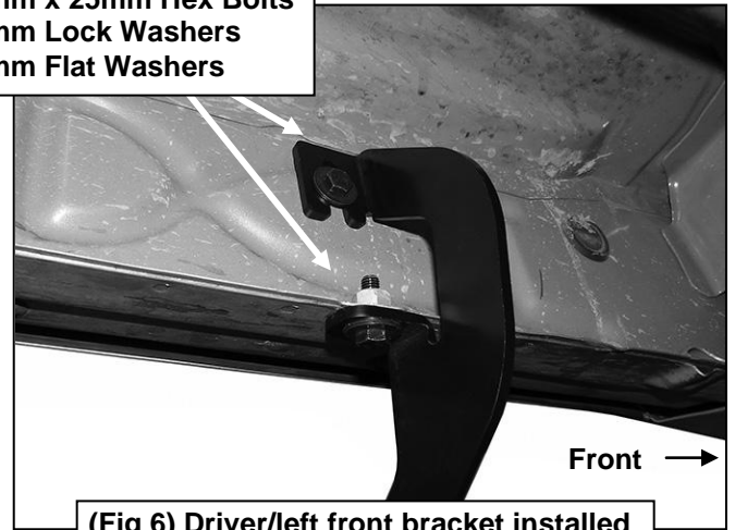
(Fig 6) Driver/left front bracket installed
