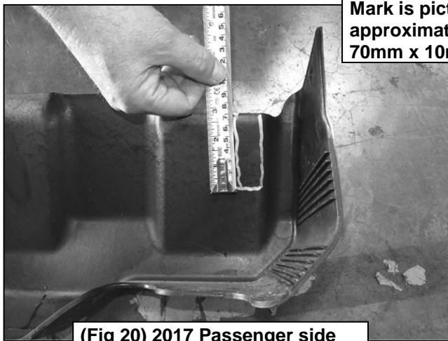
(Fig 20) 2017 Passenger side DEF cover marked for trimming
