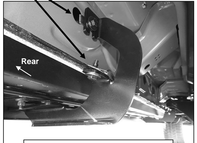
(Fig 10) Driver/left brackets installed
