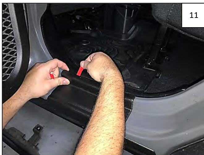
Repeat for other tape leaders from door sill areas. Do not peel tape from underside of part yet. Press part against vehicle in both sill areas.
