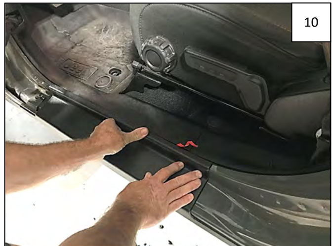
After pulling a few inches, press part firmly at area of tape before proceeding, to maintain position.
