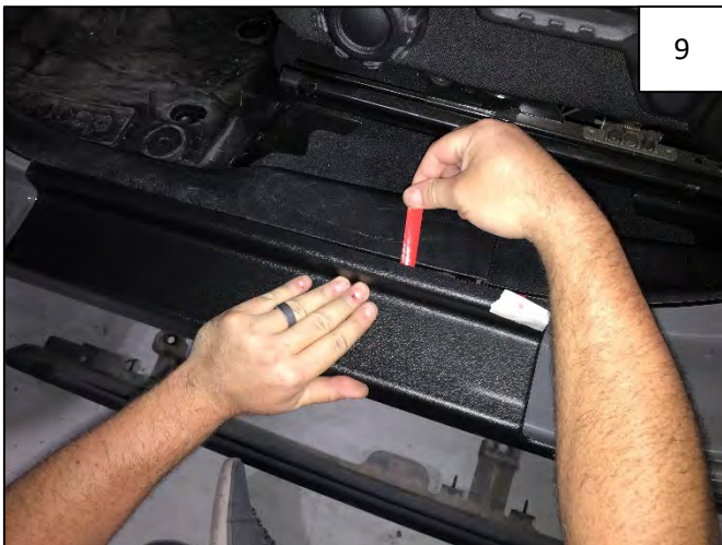
Carefully pull red tape leader marked #1 at a 45-degree angle away from part into interior of vehicle to release from the tape, pressing against part as you go. Press down on door sill before peeling next tape leader.
