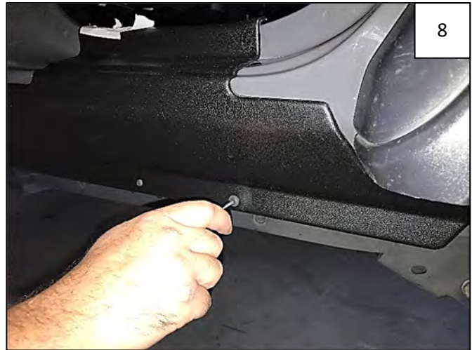
Hold part in place on door sill, and install 1 supplied #10 screw into rearmost clip installed in Steps 6-7. This will help hold the part in place for the next steps – do not tighten. Do not press the part down at areas of tape.
