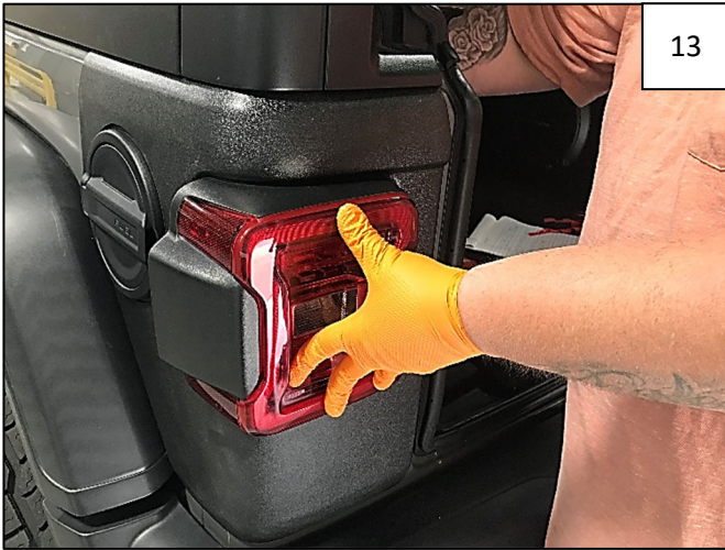
Reinstall taillight connector and taillight housing using white plastic bolt/spring you removed in Step 4. Reinstall plastic access panel removed in Step 3.
